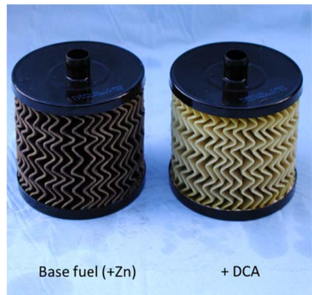
Figure 14. Fuel filters from DW10B engine test on fuel containing Zn neodecanoate with and without novel deposit control additive.
