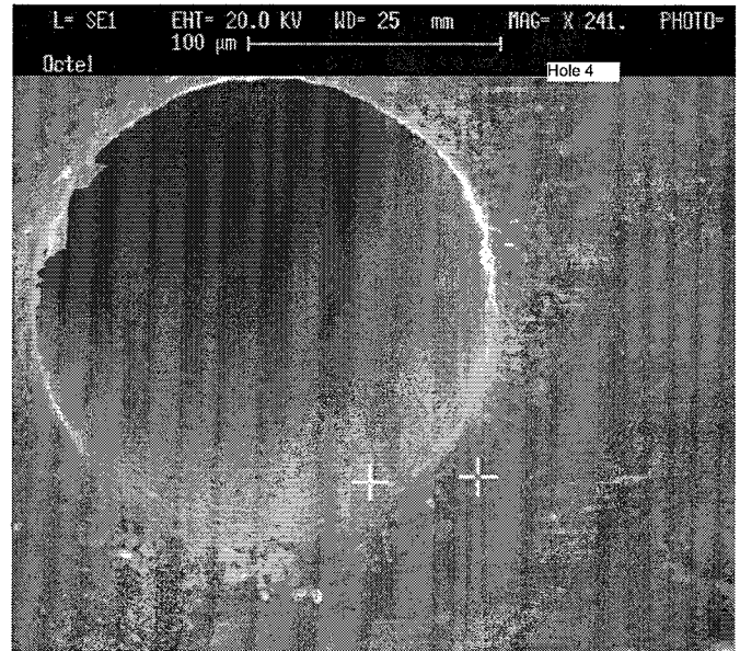
Figure 12 Hole of injector using F1.
