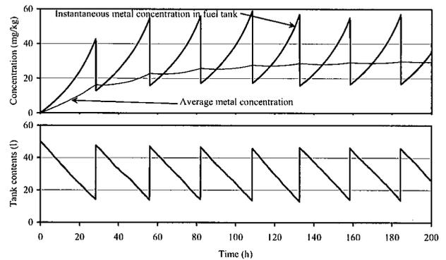
Figure 2. Simulation of low duty operation.
