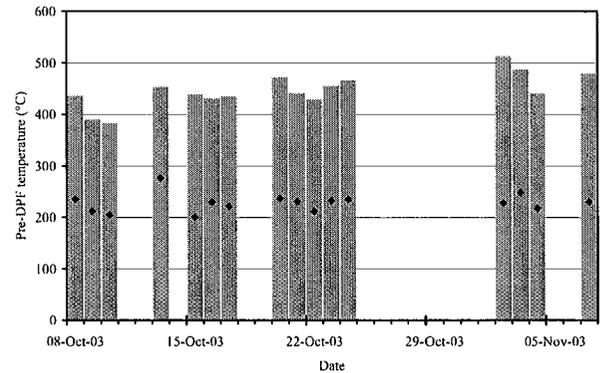
Figure 12. Mean and maximum pre-DPF temperatures per fill for Metrobus #1
