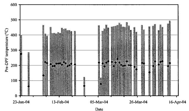
Figure 13. Mean and maximum pre-DPF temperatures per fill for Metrobus #2
