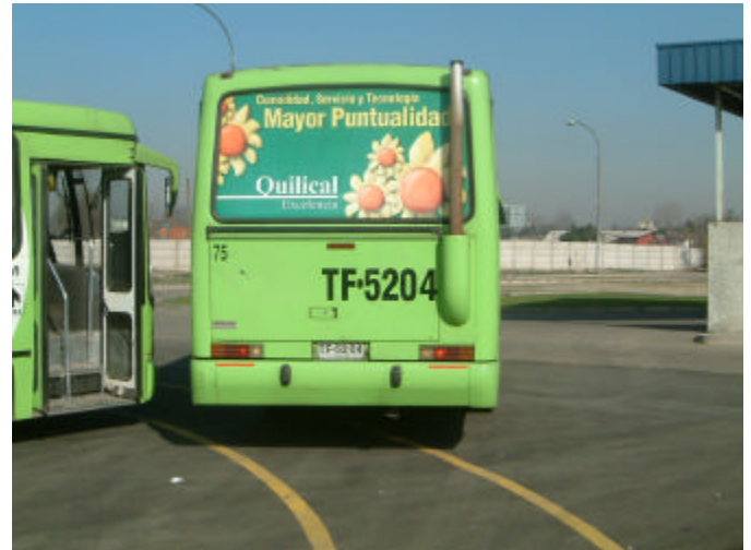
Figure 3. High level exhaust exit.
