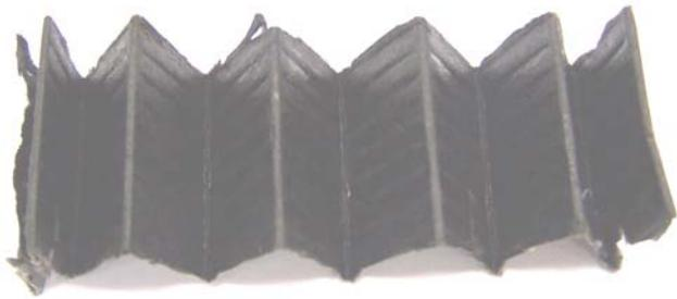
Figure 2. Typical example of a section of fuel filter
