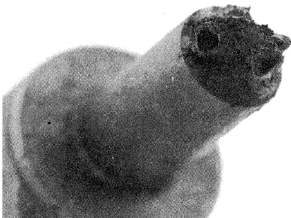
Figure 1. Deposit formation when running on peanut oil [20].
