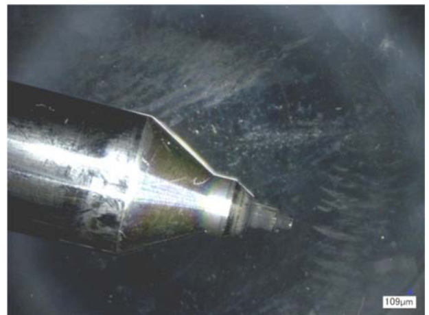
Figure 15. XUD-9 A/L injector pintle from the high treat rate PIBSI Lab1 test
