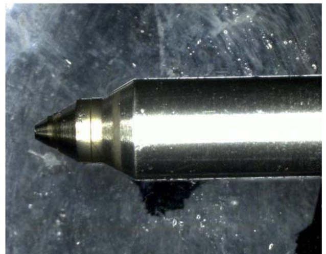
Figure 18. DW10B injector from the test with PIBSI Lab1
