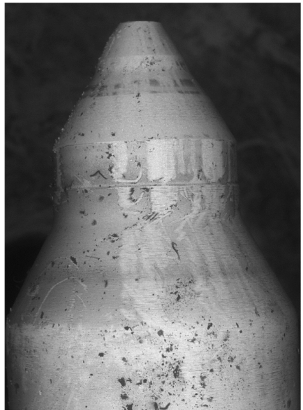
Figure 16. SEM of needle after using mono-acid lubricity improver (A3) and sodium 2-ethylhexanoate.
