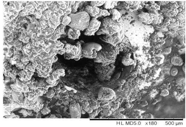
Figure 10. SEM micrograph of hole in injector 1 nozzle
