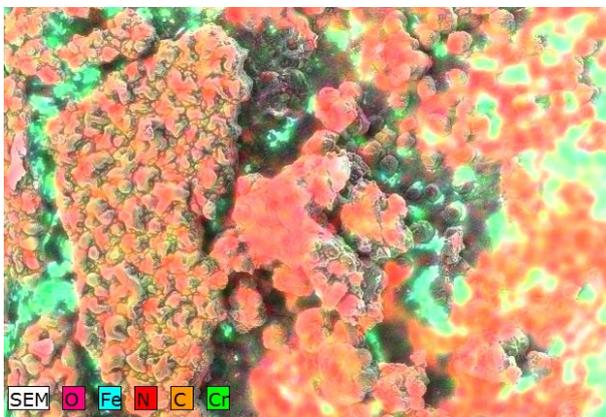
Figure 17. Elemental distribution mapping of C, O, Fe, Cr and N on region of injector 1.
