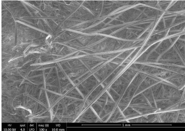
Fig. 5 SEM image of a clean filter, Sample 1.
