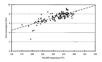
Figure 9. Average volumetric fuel consumption rate per fill
