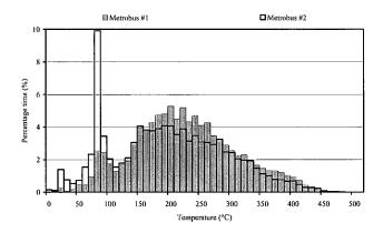
Figure 11. Pre DPF temperature distribution for Metrobuses
