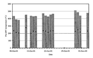
Figure 12. Mean and maximum pre-DPF temperatures per fill for Metrobus #1
