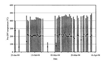
Figure 13. Mean and maximum pre-DPF temperatures per fill for Metrobus #2
