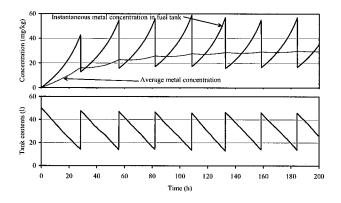
Figure 2. Simulation of low duty operation.
