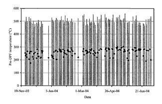
Figure 8. Mean and maximum pre-DPF temperatures per fill.
