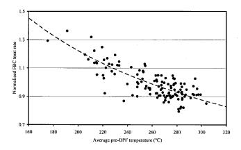
Figure 10. Relationship between FBC concentration and mean pre-DPF temperature.
