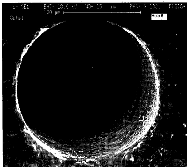
Figure 8. Injector deposits running on B100
