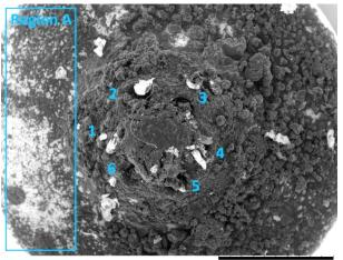
HL MD8.3 x30 2 mm Figure 20. SEM Micrograph of injector 2 nozzle tip
