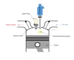
Figure 3 Gasoline Direct Injection (GDI) System
