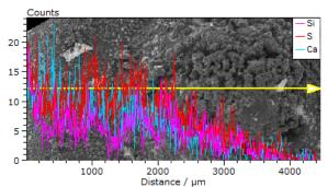
Figure 16. Linear EDS scan for detection of Si, S and Ca across a region of injector 1
