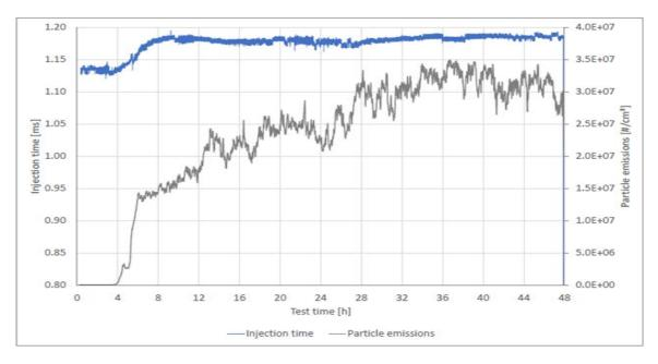
Figure 41 Increase in particle emission over length of test
