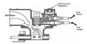
Figure 1 "Throttle Body" (TBI) Fuel Injector System
