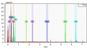
Figure 15. EDS spectrum of injector 1 nozzle tip
