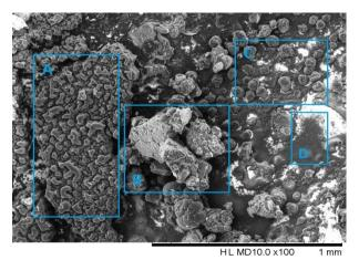
Figure 12. SEM Micrograph of injector 1 deposits
