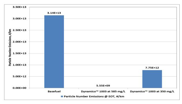
Figure 42 Effect of additization on PM emissions
