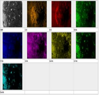
Figure 27 EDS map of injector 2 Surface.
