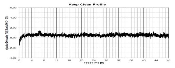
Figure 39 GDI testing keep-clean additized fuel
