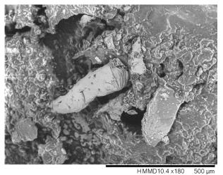
Figure 22. Mixed SEM Micrograph of hole 4 in injector 2 nozzle
