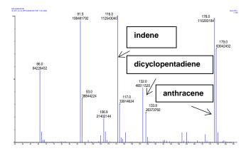
Figure 30 Positive ion APPI mass spectrum for a mixture of isoprene, indene, dicyclopentadiene and anthracene mixture.
