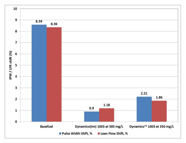
Figure 40 the demonstration of reduced injector fouling in a euro 6 vehicle with us of new generation GDI DCA additive.
