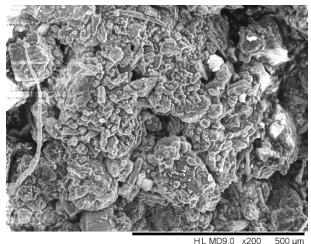
Figure 25. SEM Micrograph of injector 2 deposits
