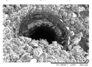
Figure 11. SEM Micrograph of hole in injector 1 nozzle
