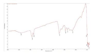
Figure 19 Infra-red Spectrum near Injector 1 Orifice.
