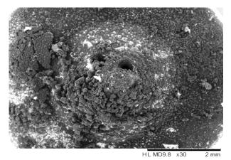
Figure 9. SEM Micrograph of injector 1 nozzle tip
