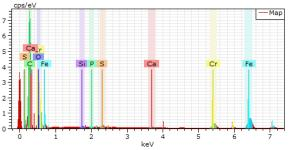
Figure 26. EDS spectrum of injector 2 nozzle tip
