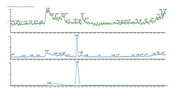
Figure 29 (top) UHPSFC +ve-ESI MS (base peak ion current chromatogram) BPICC of Gasoline used in injector 2. (middle) UHPSFC+ve ESI MS of gasoline used in injector 2 spiked with dicumyl peroxide. (bottom)UHPSFC+ve ESI MS (selected ion recording) SIR for *m/z* 119 BPICC of gasoline used in injector 2 spiked with dicumyl peroxide.
