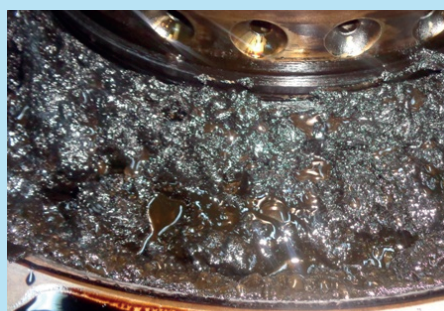
Distillate Distillate aging, polymerisation and fuel instability
