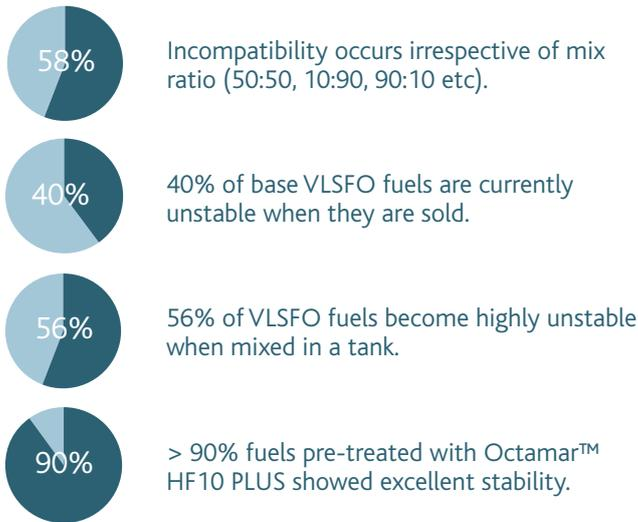
A sample ISO 8271 compliant fuel is mixed with itself and five other samples in a 90:10 ratio to test for both stability and compatibility. All six fuel samples had a high risk of instability. When tested with the same fuel samples treated with Octamar™ HF-10 PLUS every fuel combination tested positive with no risk of instability. For full test results visit [innospecinc.com/IMO2020](http://innospecinc.com/IMO2020).
