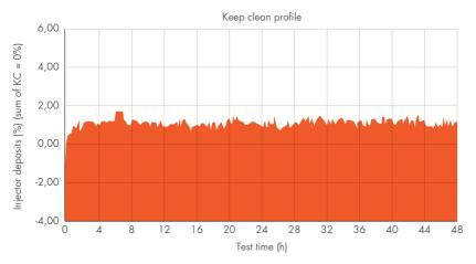
GDi keep clean testing with Dynamico<sup>TM</sup> demonstrating no increased injector fouling over test duration and excellent deposit control.
