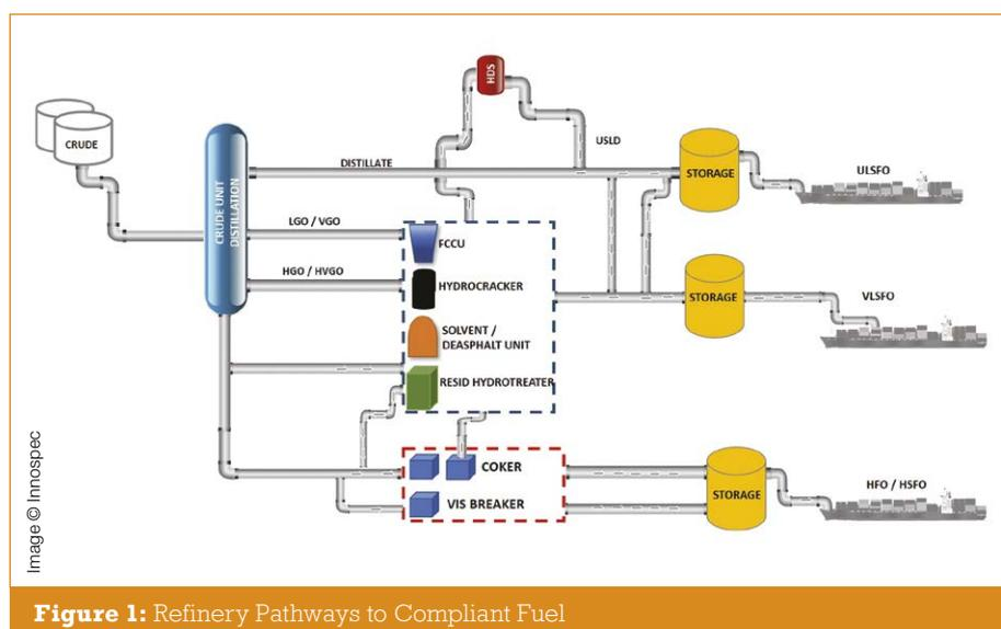
Figure 1: Refinery Pathways to Compliant Fuel
