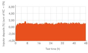
GDi keep-clean testing with Dynamico demonstrating no increased injector fouling over test duration and excellent deposit control.
